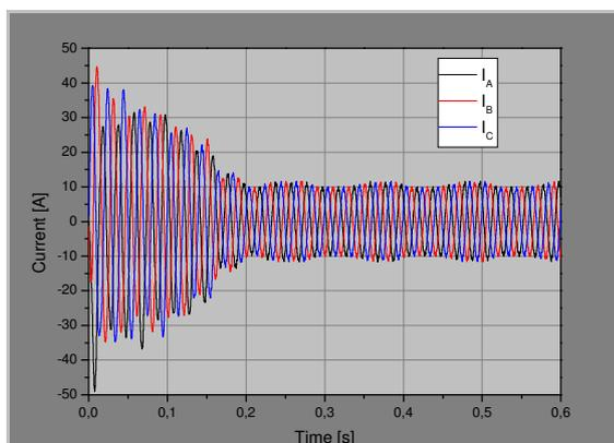
Fig. 7 Current-time variation, 5 broken bars
