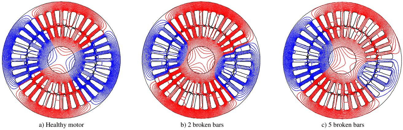
Fig. 2 Flux lines distribution
