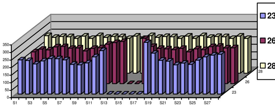
Fig. 1 Rotor bar current distribution for healthy motor (28), two broken bars (26) and five broken bars (23)
