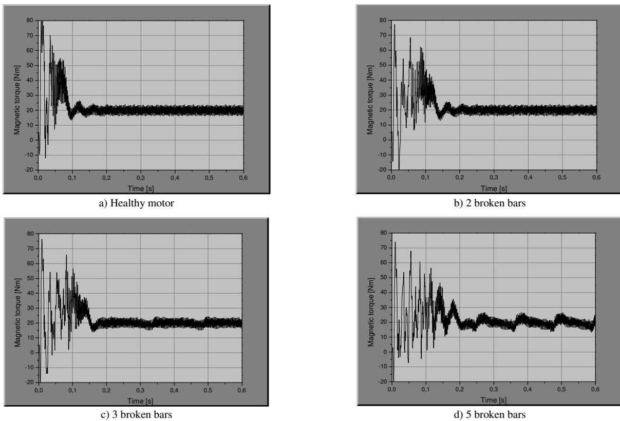
Fig. 4 Torque variation during start-up
