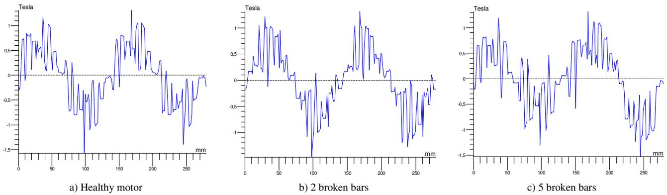
Fig. 3 Air-gap flux density
